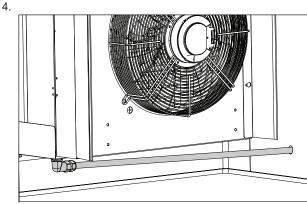
G.4.4 Inserting the trolley tray rack in appliances
