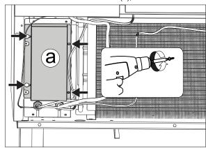
Connect the power cable (EI) as shown in the figure below, following the electrical wiring diagram included in the appliance;
