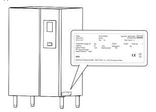
In **20GN 2/1** models the dataplate is located on the upper part of the left side of the appliance. The plate giving the appliance PNC code and serial number is located on the top of the appliance.
