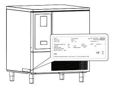
In **20GN 1/1** models the dataplate is located on the lower part of the right side of the appliance. The plate giving the appliance PNC code and serial number is located on the top of the appliance.
